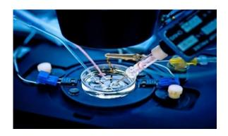
The electrophysiological behavior of neurons is studied in a 12-patch clamp as shown in figure 6 especially designed for this Blue Brain project. Twelve numbers of living neurons are synchronously patched and their electrical activities are recorded.
